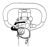
Figure 15. Throttle Lever ((Fast)
